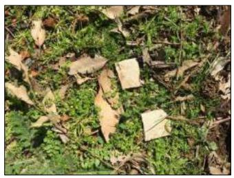
Plate 19 – Fragment of ACM observed associated with demolition waste near the dam.
